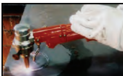
Attachment for small circle cutting ø 30mm - ø 200mm (1 1 / 4 -8in)
