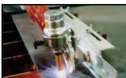
Guide rail for straight line cutting
