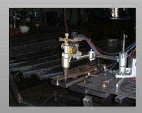
**Easy Tip Replacement:** The tip can be easily cleaned and replaced. Flame adjustment is made easy by simply raising the tracer head.
