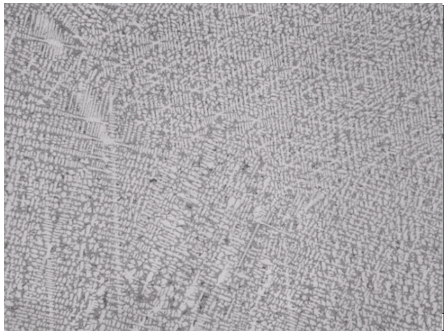
Optical Micrograph of a Stellite® 12 PTA Deposit at 500X.
