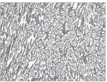
Optical micrograph of a Stellite ® 1 weld overlay
